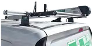
We offer a wide range of accessories for our roof bars. A rear roller will facilitate loading and unloading whilst protecting the rear of the vehicle, side load stops will keep your cargo secure and lashing eyelets and hooks offer smart lashing possibilities.
